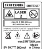
The CMHT77637 tool emits a visible laser beam, as shown in Figure A ①. The laser beam emitted is Laser Class 2 per IEC 60825-1 and complies with 21 CFR 1040.10 and 1040.11 except for deviations pursuant to Laser Notice No. 50, dated June 24, 2007.
